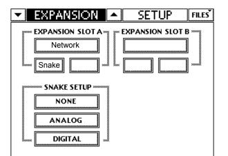
3. When the DS3232 is powered on and properly connected, "Snake" should appear under "Network," with Snake Setup options for NONE, ANALOG, or DIGITAL.
